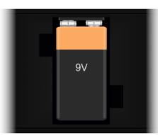
Make sure the positive and negative battery terminals are inserted correctly
